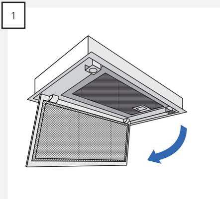
1 Open the door by pulling down on the edge of the glass plate that faces the Thermex logo on the hood.
