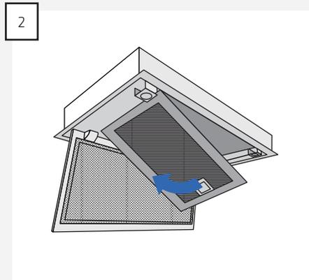
2 Remove the grease filter by pulling on the filter locking mechanism to loosen the filter from the hood.
